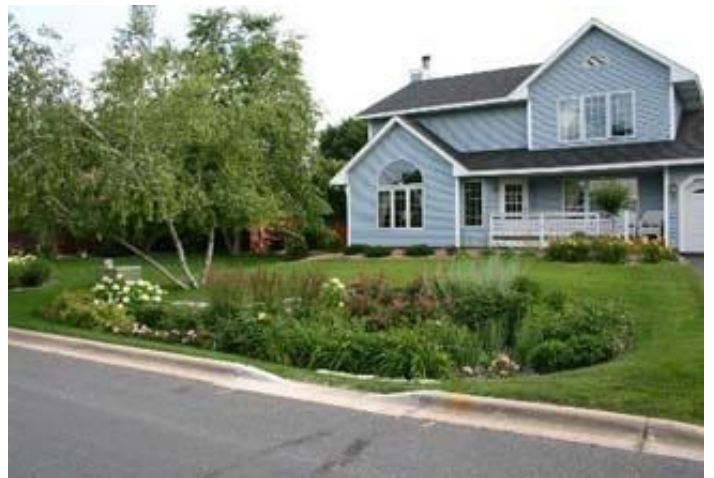
Rain gardens reduce runoff while adding a landscaping element. Source: epa.gov/green-infrastructure
