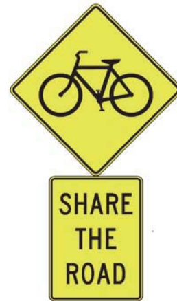
Figure 10: "Share the Road" Signs Source: MUTCD, Part 9
