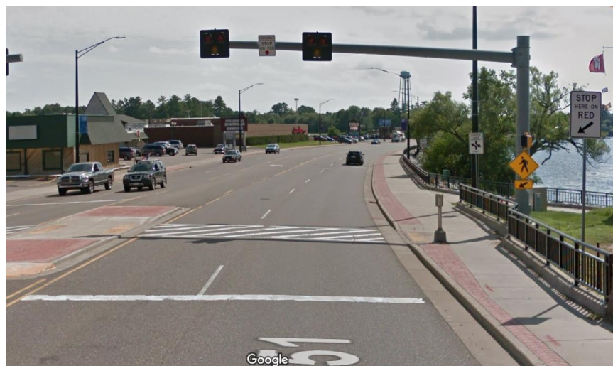
High-intensity Activated Crosswalk (HAWK) in Minocqua
