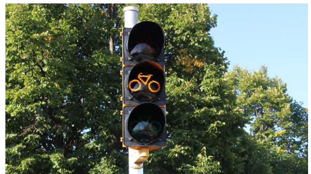
Figure 4-9: A bicycle signal head can be used at a crossing where a hybrid beacon is used Source: Nacto.org
