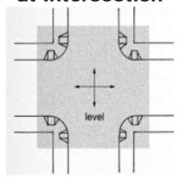
The preferred design is to have a separate curb ramp aligned with each crossing direction to allow all pedestrians to cross at the same location. At most intersections, a pair of perpendicular curb ramps placed at 90 degree angles to one another is the optimal design for meeting these criteria.
