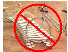
Racks that hold the bike by the wheel with no way to lock the frame and wheel to the rack with a U-lock
