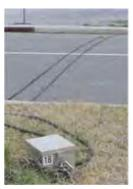
can provide basic traffic counts and average traffic statistics. The equipment can also provide vehicle classification statistics whether it is a car or a trunk and even what type of truck. Traffic may also be broken down by time of day. Speed statistics are also possible which may be of assistance in setting speed limits or identifying speeding trouble spots.
