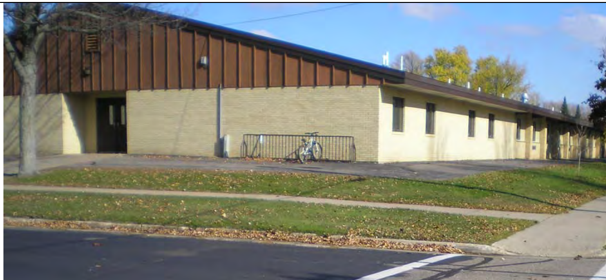
Good bike rack location, because it is near an entrance, and is accessible on a paved surface.
